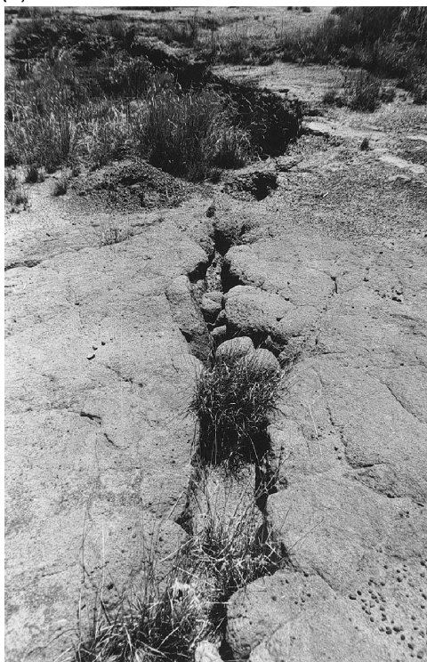
Fig. 4. (a) Subsidence due to pillar failure. (b) Tension fracture developed in sandstone running away from an area of subsidence due to pillar failure.
